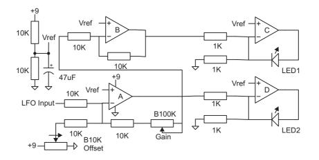
This circuit takes an LFO input and converts it into lighting two LEDs. One LED gets brighter as the other gets dimmer, and vice versa.
